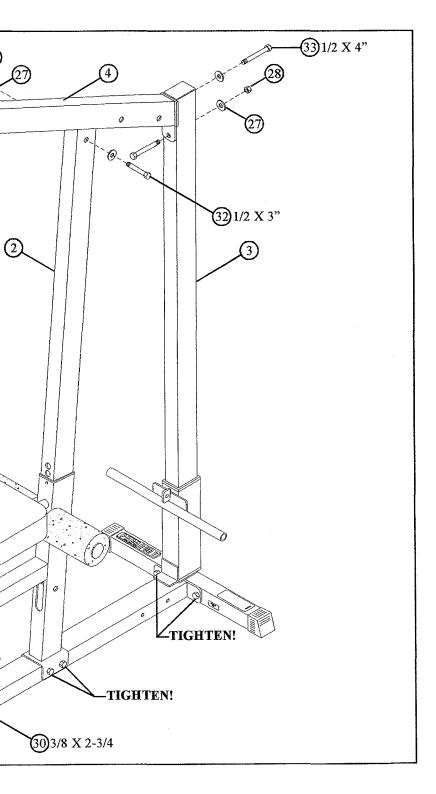
• LOOSELY assemble the TOP BOOM (4) to the FRONT UPRIGHT (2) using one 1/2 X 3" BOLT (32), two 1/2" WASHERS (27),
